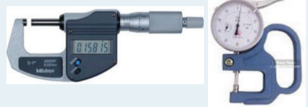
FIGURE 5. Digital micrometer for measuring hair shaft diameter (left); thickness gauge for measuring hair shaft diameter (right).
